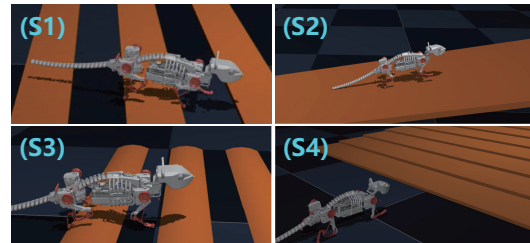
Fig. 5. Four test scenarios for the rat robot. (S1)Planks: Gallop over planks with wide gap(width=10 cm).(S2)Uphill: a 10-degree slope. (S3)Logs: Upon a pile of logs. (S4)Stairs: Micro stairs between two platforms.
